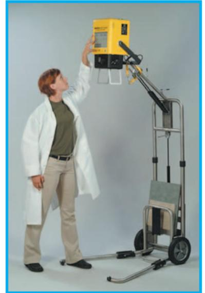
... and unfolds easily to position focal spot as high as 76" above the floor.
